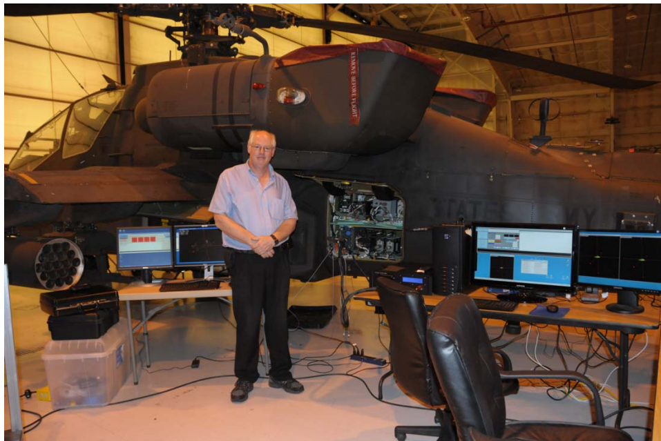
Real Threat Emulator injecting INS, IMU, and UV Threat Profiles into an Apache AH64D Aircraft (official photo release)
