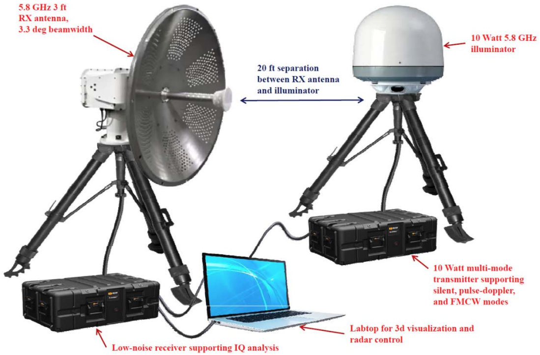
Silent Multi-Mode Radar supporting FMCW, Pulse-Doppler, and "Silent" modes of operation
