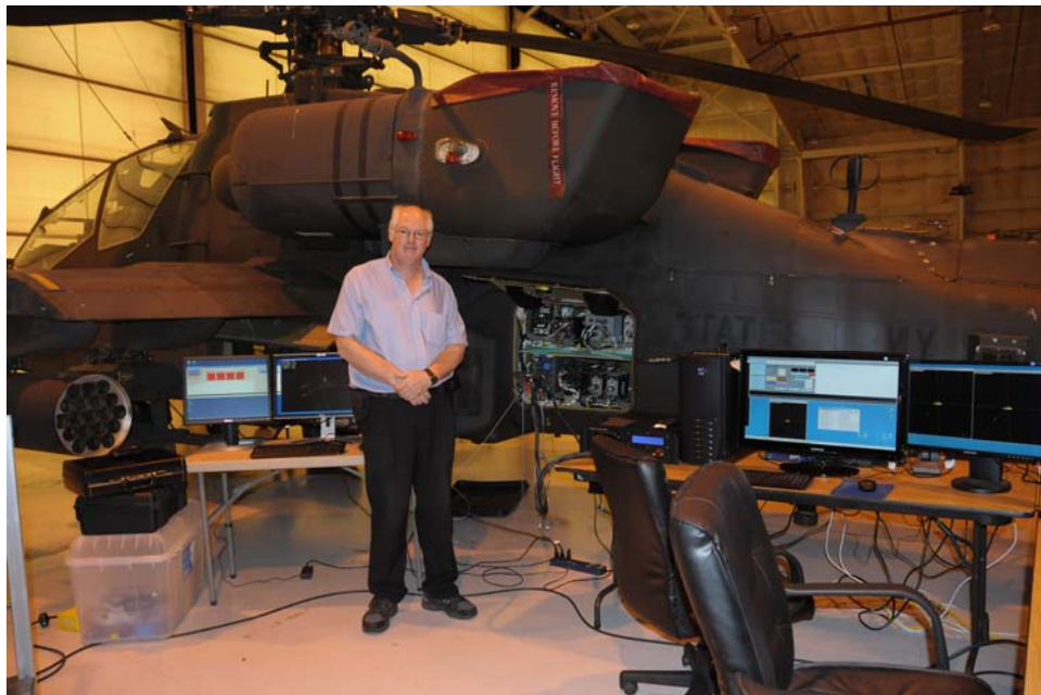
Real Threat Emulator injecting INS, IMU, and UV Threat Profiles into an Apache AH64D Aircraft (Unclassified)
