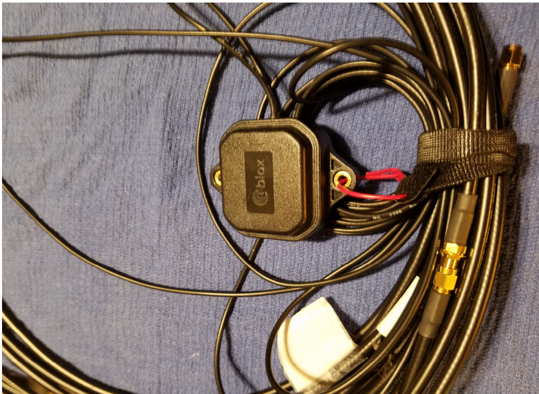
Figure 6. Ublox ANN-MB series precision GNSS active antenna
