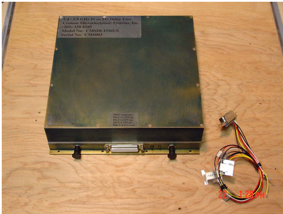
Figure 6. Fiber-Optic Delay Line for Korean Radar Calibration System
