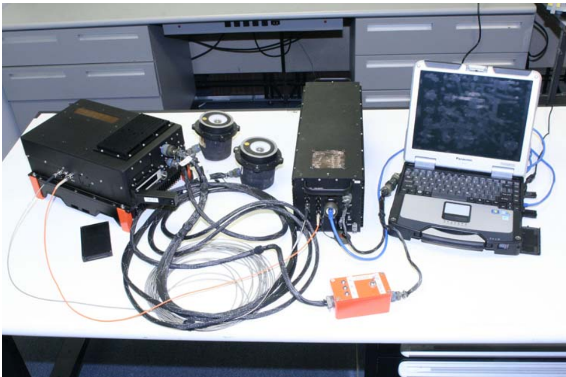
Figure 25. CIDR-DAU System (External View) (System activates EOMS UV sensors from the Common Missile Warning System)
