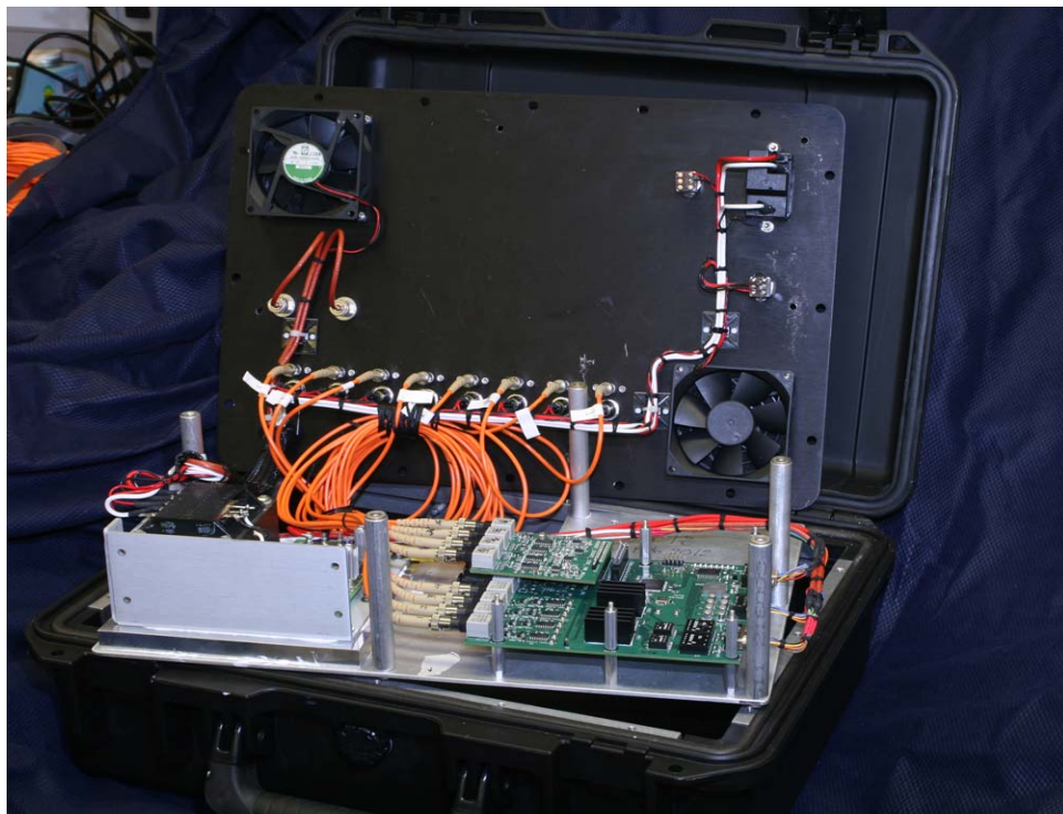
Figure 23. Field Unit 1553/1773 Fiber-Optic Transceiver for AMRDEC (External View)
